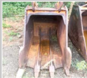
KOMATSU PC200 TRENCHING BUCKET
