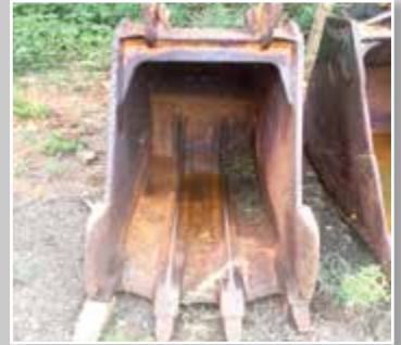
KOMATSU PC200 TRENCHING BUCKET
