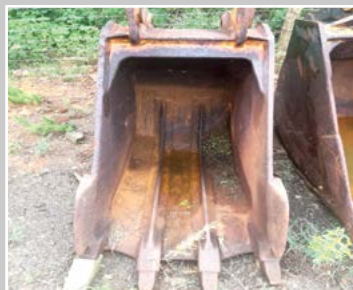
KOMATSU PC200 TRENCHING BUCKET
