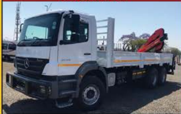
2006 Mercedes Benz 2628 LWB fitted with Dropside Body and Palfinger PK12000 Rear Mount Hydraulic Crane.
